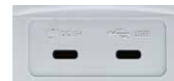
2 x type C USB port Power port / Data port
