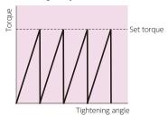
A clear 'Rotary-slip' shake signals tightening completion upon reaching the set torque. The shock repeats if tightening after reaching the set torque continues. Because users can tighten no further than the set torque, over-torque is completely prevented.
